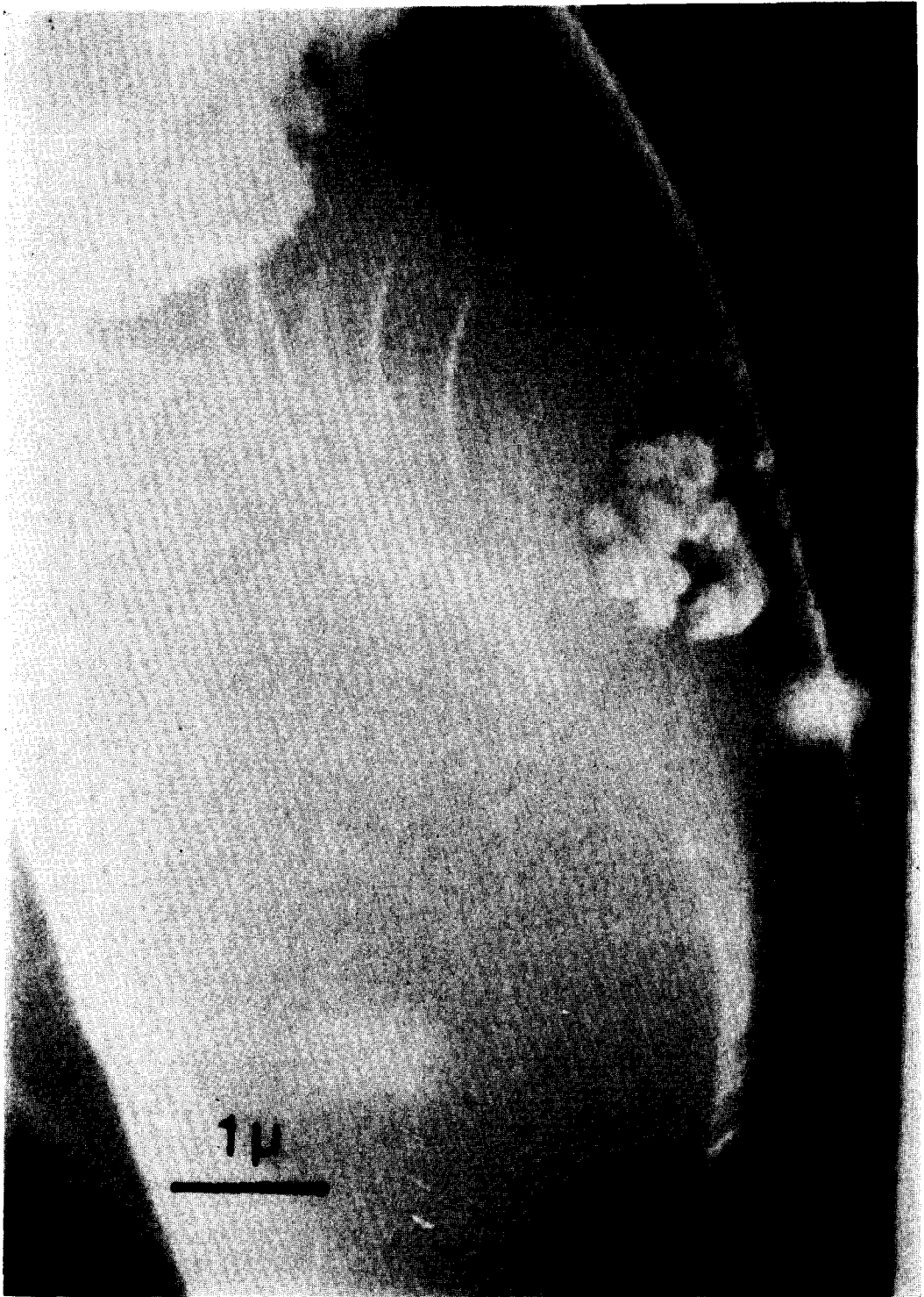
FIG. 2. Scanning electron micrograph of La 2 O 3 starting material.
